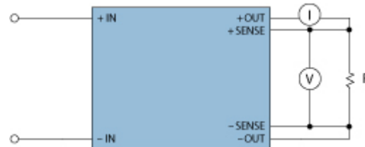
Figure 7b Detail of load regulation measurement circuit
