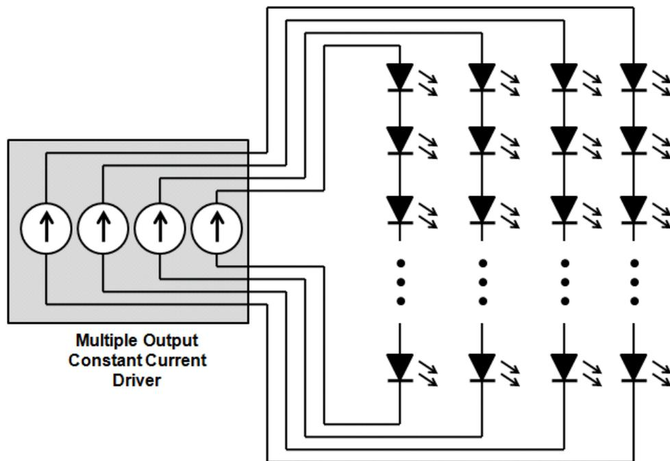
Figure 4: Multi-Channel Configuration
